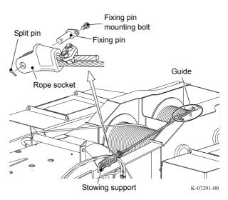
**9.** Wind up the auxiliary winch until the auxiliary wire rope is tensioned slightly.
