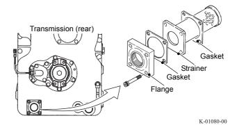
**4.** Immerse the strainer in volatile solvent such as kerosene, and clean it with a soft tool such as nylon brush.
