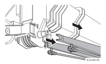
**14.** Direct the right and left jib set pins from the bottom to the top to insert, and fix them with the snap pins.
