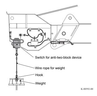
**8.** Hoist up the auxiliary wire rope, and make the auxiliary hook block slightly contact with the head of the jib.
