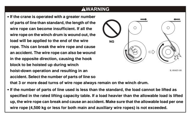
If the over-unwinding cutout function (option) is provided, the winch winding down operation is stopped automatically when the remaining number of dead turns of wire rope reaches approx. 3.
