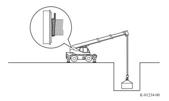
• Do Not Suspend Loads for a Long Time Avoid keeping a load lifted for a long time. Arrange the work procedure to minimize the load-lifting time.
