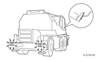
**4.** Check that the backup lamps light up when the shift lever is set to "R".
