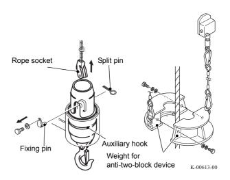
**34.** Remove the pin from the rod of the switch for the anti-two-block device, and mount the weight for the anti-two-block device and the wire rope for the weight, so that the anti-two-block device for boom lift can be activated.
