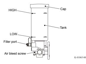
bleed screw. When air is no longer contained in the discharged grease, tighten the air bleed screw and tighten the filler port cap.
