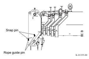
**12.** Install the bolts on the main hook block.
