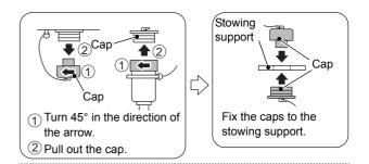
Anti-two-block device connector
