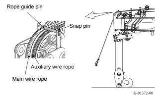
(10)Attach the rope guide pin for the upper sheave of the top boom section.
