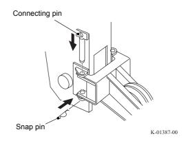
6. Insert the pin through the rod of the switch for anti-two-block device, and remove the weight for the anti-two-block device and the wire rope for the weight, so that the anti-two-block device for boom lift does not activate.
