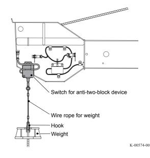
Disconnect the wiring for the anti-two-block device between the top jib and base jib. Attach the cap to the removed connector for the extension wiring and stow it into the stowing position.
