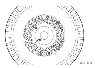
**10.** After a tire is replaced, tighten the wheel nuts again with the specified tightening torque after approximately 50 km of traveling.
