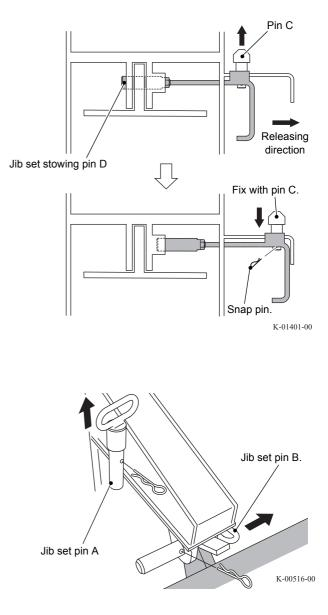
**11.** Pull the jib set pins A and B.
