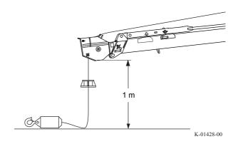
Disconnect the connectors for the anti-two-block device on the jib head. Attach the cap to the removed connector for the anti-two-block device, and remove the wiring from the guide.
