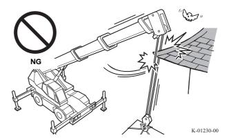
• Carefully Operate While the Boom is Raised High When the boom is raised close to its upper limit angle, the horizontal clearance between a lifted load and the boom becomes small. If the lifted load sways in this condition, the load can collide with the boom or jib. This can damage the boom or jib, or the load itself. Carry out operation carefully when the boom is raised close to its upper limit angle, so that the load will not collide with the boom or jib.
