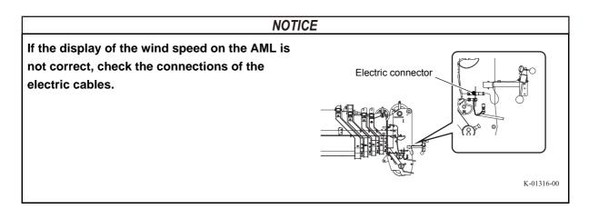
The anemometer measures the wind speed at the boom or jib head in order to prevent damages to the crane or an overturning accident caused by a strong wind.
