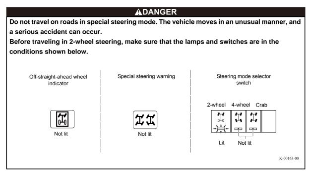
The example here explains the steps for changing the 4-wheel steering mode to 2-wheel steering mode.
