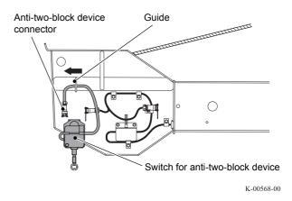
**12.** Connect the connectors for the anti-two-block device.
