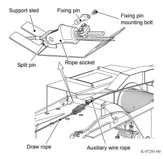
(3) Wind out the auxiliary wire rope while pulling the draw rope from the front of the boom.
