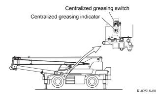
**2.** When half of the greasing cycle is completed, the indicator goes out, and the grease pump stops.
