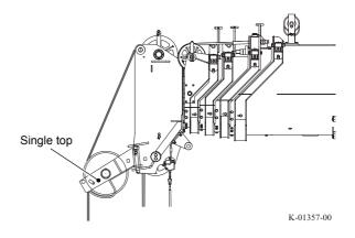
8. Connect the connectors (2 points) for the anti-two-block device.
