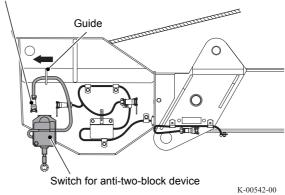
39. Connect the wiring of the switch for the anti-two-block device and extension wiring to connectors on the top jib.
