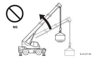
gravity center, the load does not stick to the ground or does not touch other loads or structures. Lift up a load vertically, and stop lifting again when the load is raised by several centimeters above the ground and stop the sway of the load. Check that the state of rigging is fine, the load is securely held at the position, and the machine is not overloaded. And then, lift up the load again.
