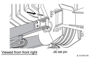
**15.** Pass the provided guide rope between the sheave on the jib head and the guide pin, and attach its end to the support on the boom.
