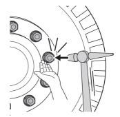
Tap lightly in a direction which the wheel nut is tightened.
