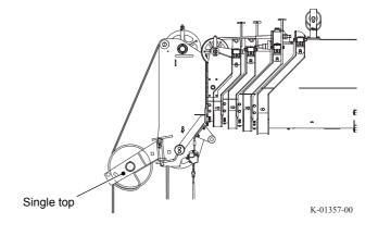
**9.** Mount the rope socket in the orientation as shown in the illustration.
