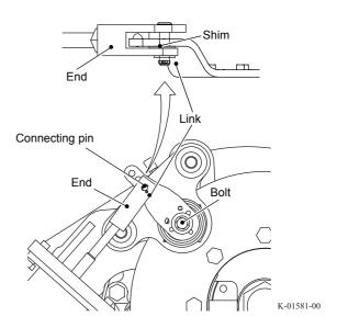
**5.** Turn the link 4 pitches clockwise so that the sum of the clearances between the pad and disc plate is  $0.7 \text{ mm} (\pm 0.1 \text{ mm})$ .
