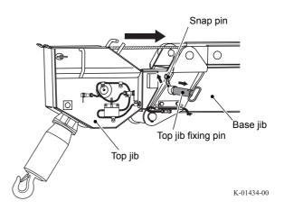
**8.** Slowly unwind the auxiliary wire rope to extend the top jib.
