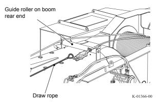
(2) Attach the draw rope and support sled to the rope socket of the auxiliary wire rope.
