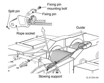
8. Remove the rope guide pin for the upper sheave on the top boom section, and pass the provided draw rope.
