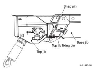
**10.** Attach the switch for anti-two-block device at the jib head, and pass the wiring for the anti-two-block device through the guide.
