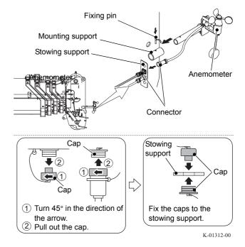
**2.** Install the anemometer to the mounting support on the jib head and fix it with the fixing pin.
