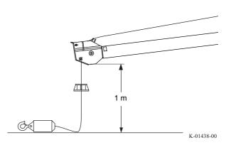
**3.** Disconnect the connectors for the anti-two-block device on the jib head. Attach the cap to the removed connector for the anti-two-block device, and remove the wiring from the guide.
