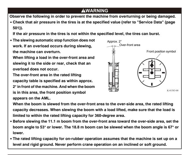
**NOTICE** The machine is supported by the tires in on-rubber operation. The load can easily sway due to deflection of the tires. Operate the crane slowly and safely.
