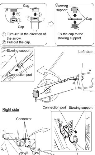
Dummy plug stowing support K-01390-00
