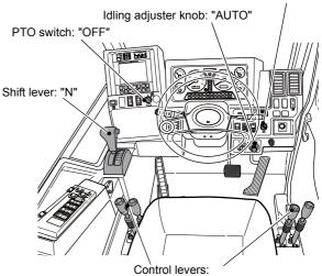
Return to the neutral position, and then lock and set to the stowing position K-04846-00
