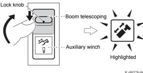
Boom telescoping/auxiliary winch
