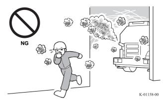
• Stop the Engine during Inspection and Maintenance
