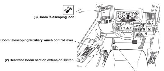
Boom telescoping control pedal
