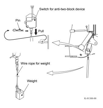
**7.** Reeve the wire rope through the sheave of the single top. Then install the anti-two-block device and the weight for anti-two-block device to the single top.
