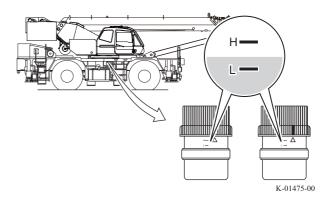
If the brake fluid level is low, check for any fluid leakage in the piping system. Remove the cap on the brake fluid reservoir, and add brake fluid to "H" line.
