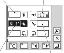
Boom angle upper limit is highlighted. Boom angle lower limit Current boom angle is displayed.
