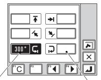
Left slewing limit is highlighted. Current slewing angle is displayed.
