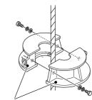
Weight for anti-two-block device
