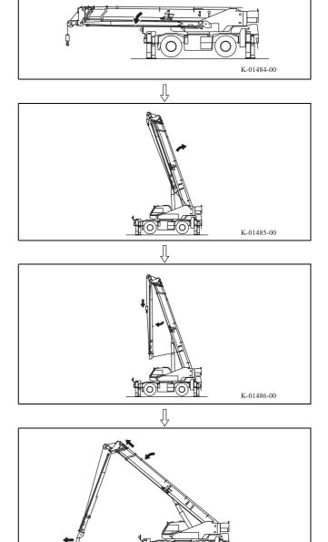
4. Extend the boom while lowering the boom, and swing the jib forward.(Steps 29 through 32)
