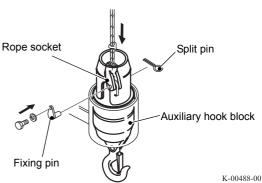
**9.** Insert the fixing pin and secure the rope socket to the auxiliary hook block.
