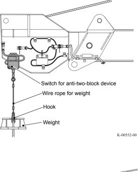
**7.** Hoist up the auxiliary wire rope, and make the auxiliary hook block slightly contact with the head of the jib.
