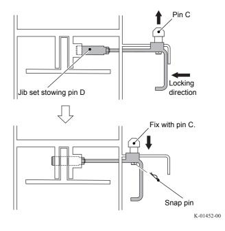
**32.** Direct the jib set pin to the boom head and insert it, and fix the jib to the boom.
