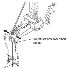
Weight for anti-two-block device
