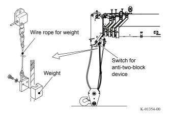
**5.** Remove the snap pins, and pull out the two rope guide pins.
