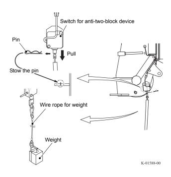
**8.** Pull out the connecting pin, and rotate the single top and stow it.
